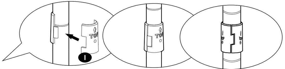
The gaps between the plastic clips are a structural design rather than a quality issue, making it so the clips can be firmly anchored to the tubes and easily disassembled as you need.
