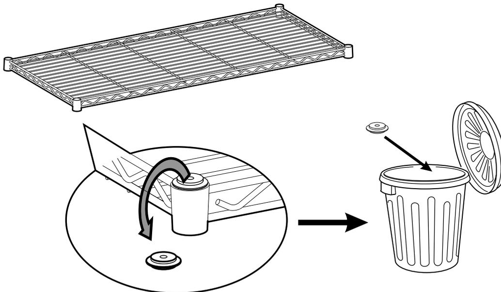
The plastic covers on the cone sleeves are to protect the product during transport. Remove and dispose of them before assembly.
