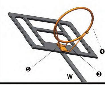
Insert ③ into slot ④, then insert ③ and ④ into the fixing block (⑤) and press it into the slot. Finally, attach the fixing block (⑤) to the backboard (⑥) and fix it to the backboard (⑥) with screws (W)
