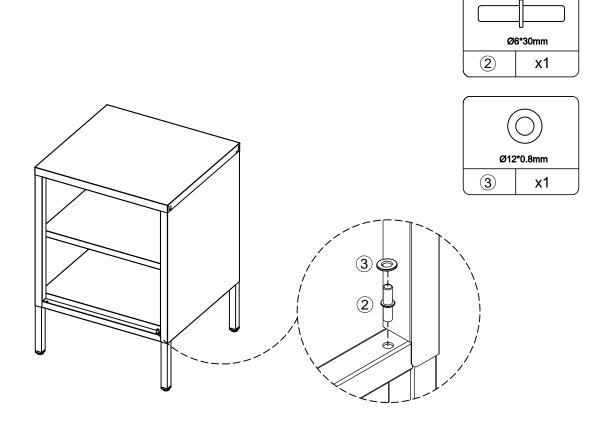
$\left(7\right)$  - Attach (C1) & (C2) to pre-assembled unit as below shown.
