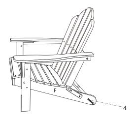
6.Attach part(G) to part (F) by using screws (4) as shown in the diagram.  $\frac{open}{concept}$
