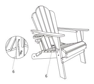
8.Use screw (6) to install the pin onto part(B)and part(C) as shown in the diagram.
