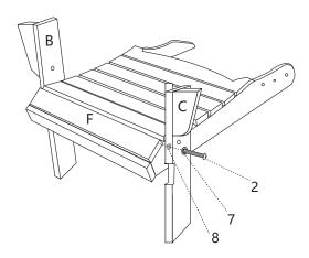
1.Attach part(B) to part (F) by using screw (2)and nut(8) and gasket(7) as shown in the diagram.
