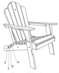
4.Attach part(I) to part (A) by using screw (4)as shown in the diagram.
