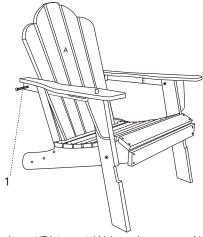
3.Attach part(D) to part (A) by using screw (1)as shown in the diagram.
