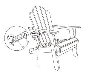
7.Attach part(J) to part (D) by using screws (10) as shown in the diagram.
