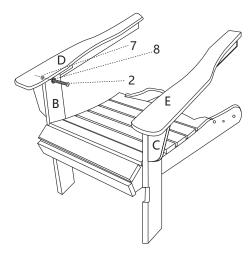
2.Attach part(D) to part (B) by using screw (2)and nut(8) and gasket(7) as shown in the diagram.
