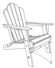
5.Attach part(H) to part (B) and part (C)by using screw (5)as shown in the diagram.
