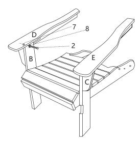
2.Attach part(D) to part (B) by using screw (2)and nut(8) and gasket(7) as shown in the diagram.
