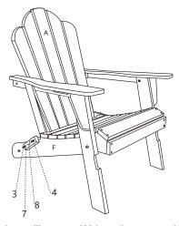
4.Attach part(I) to part (A) by using screw (4)as shown in the diagram.
