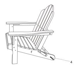
6.Attach part(G) to part (F) by using screws (4) as shown in the diagram.
