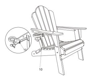
7.Attach part(J) to part (D) by using screws (10) as shown in the diagram.
