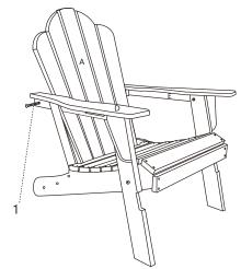
3.Attach part(D) to part (A) by using screw (1)as shown in the diagram.
