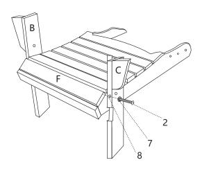
1.Attach part(B) to part (F) by using screw (2)and nut(8) and gasket(7) as shown in the diagram.
