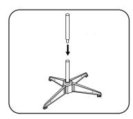
2. Insert the upper pole into the lower pole;
