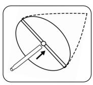
3. Make sure the top of the upper pole going through the iron hole in the middle of the base bar inside the tree;
