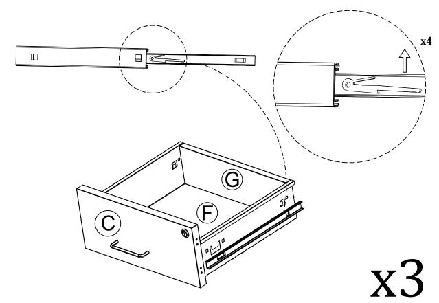
(9) -Attach Drawer to pre-assembled unit as below shown.
