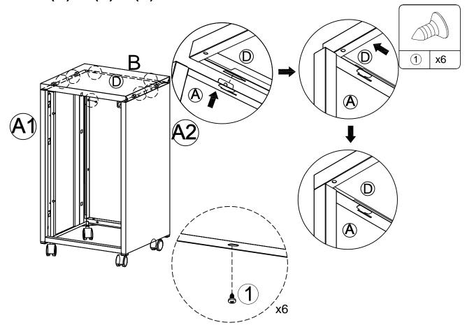
$\left(5\right)\,$  -Attach Drawer Slide Rail Shell  $\,$  to (A) as below shown.
